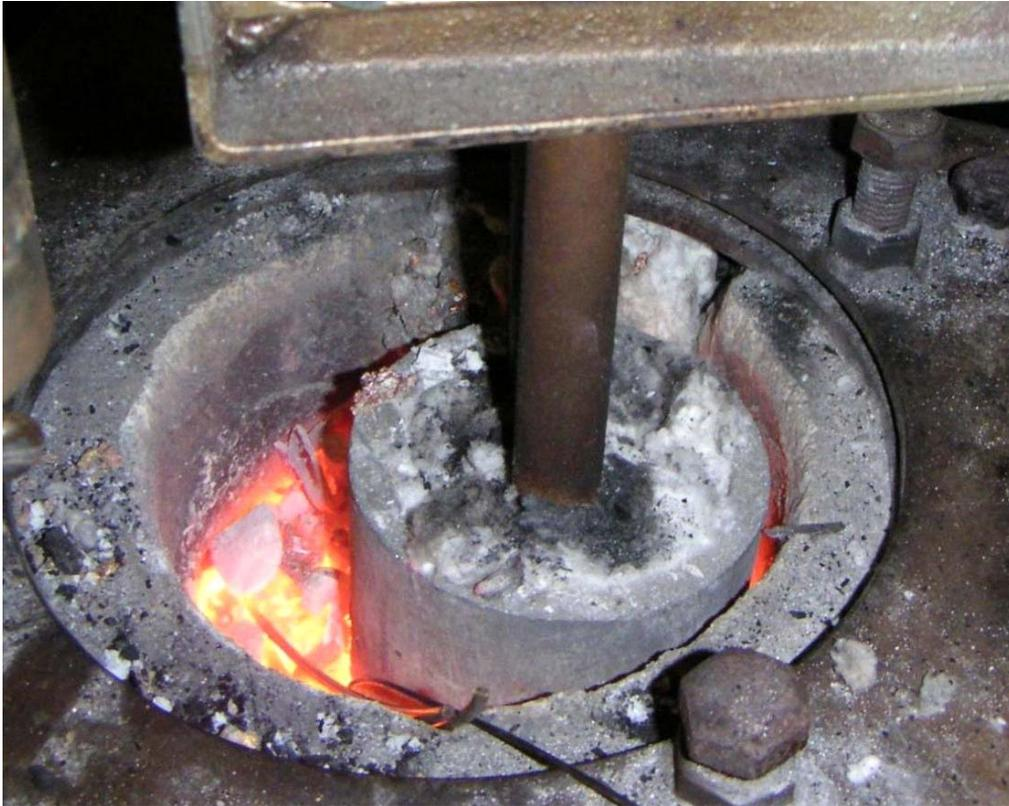
6mm wire-rod production die and cooler assembly immersed in melt-bath.
