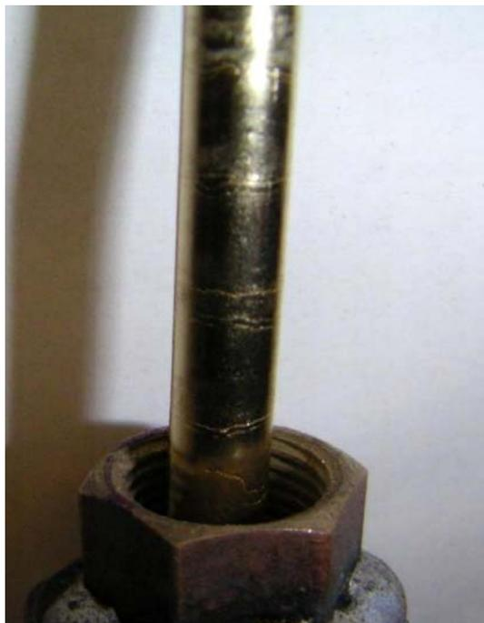
6mm dia. Wire-rod in Cu alloy casting upwards out of the the die assembly.
