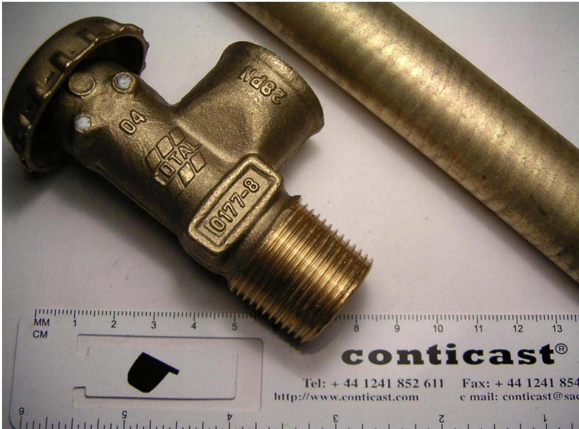
CONTICAST 37Ø as-cast C37700 brass rod (top) & an lpg cylinder valve produced there-from (lower).
