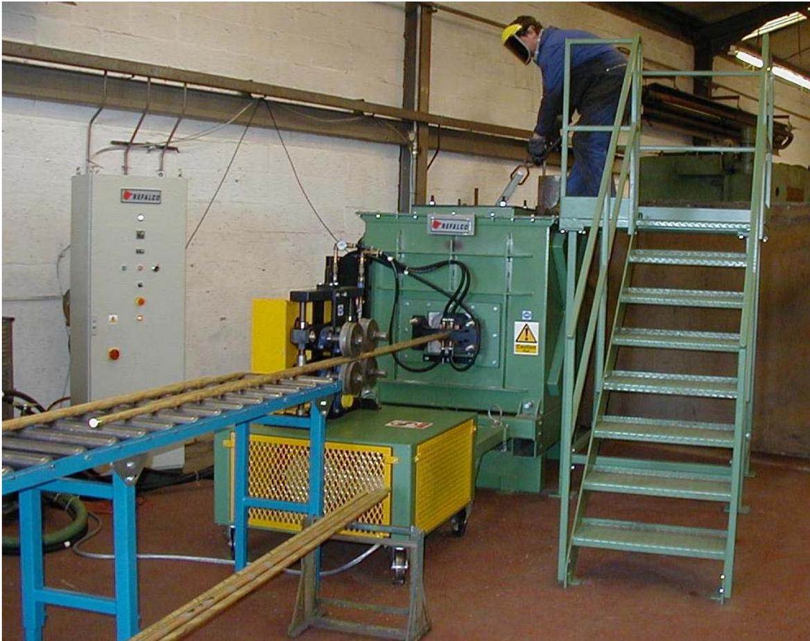
**CONTICAST CONTINUOUS CASTING MACHINE (Model RF700HCC)**
