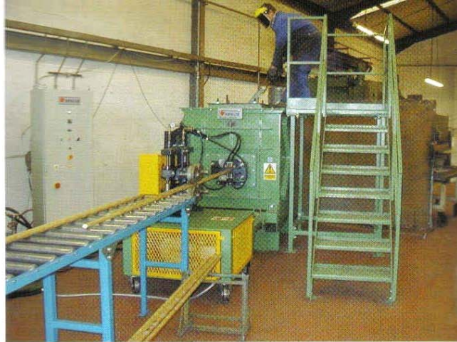
A horizontal continuous casting machine in operation producing twin strands.
