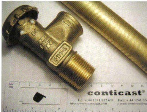
An LPG valve produced by logging and machining. The conticast brass bar is the raw feedstock.
